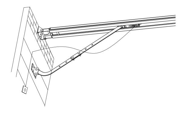
In some situations that a pedestrian door is not in state, it is recommended that an external disengagement device should be fitted.
