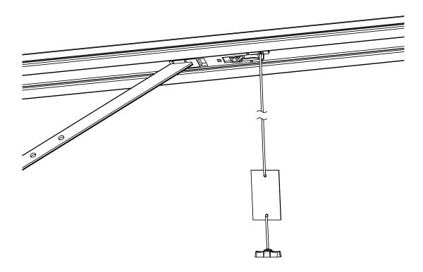
The opener is equipped with a manual release cord to disengage shuttle and move door by hand while holding the handle down. Pull on the handle to disengage the shuttle. To re-engage the door simply run opener in automatic mode or move door by hand until the trolley engages in the chain shuttle.
